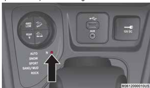
Interruptor de neutral
