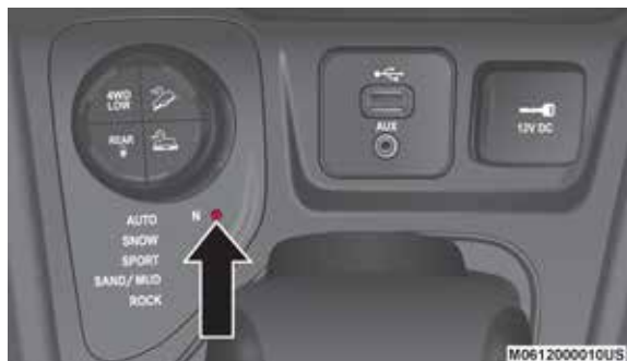
Interruptor de neutral
